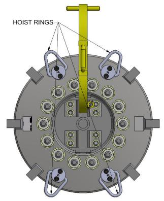
4. The Vent open end should face down if the test medium will be "siphoned" out of the system through the GripTight Test Plug port for recycling, reuse, etc. Position the Lifting Fixture in the appropriate orientation to facilitate installing in the desired orientation. The Lifting Fixture is shown in an orientation that would place the open end of the Vent up to facilitate displacing and venting air from the test pipe.
