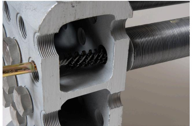
Plug Installation (Installing Pop-A-Plug® inside the tube sheet at depth)
