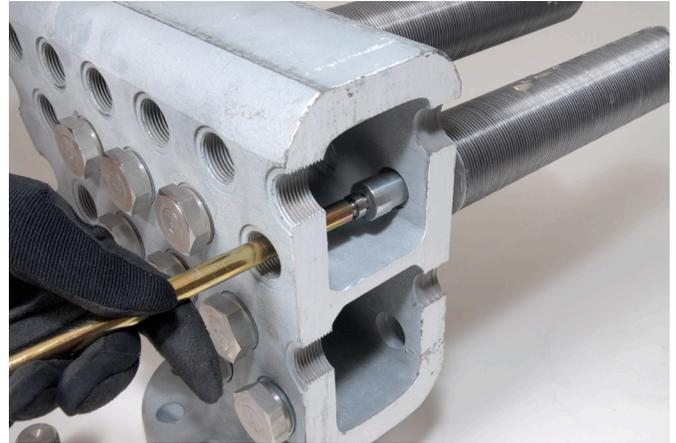
Tube Brushing (Cleaning inside of tube of scale, rust, debris etc. for a clean surface)
