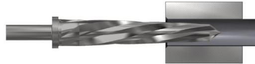
Install tapered reamer in a variable speed drill and lightly lubricate. The small end of tapered reamer should fit into tube ID and large end should not. The reamer should be operated in the following manner:
