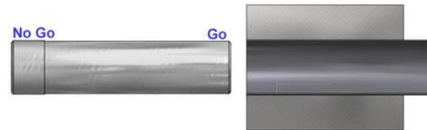
Small end of gage should fit in tube to installation depth and large end should not.
