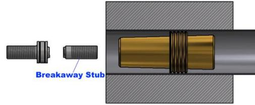
**Note:** Weeping during hydro test indicates small surface imperfections in the tube that are difficult to see. A large leak indicates a surface imperfection in the tube such as scarring from a drill used to remove a sleeve or tapered pin that should have been seen in step 5. In either case, remove Pop-A-Plug using EST Group Pop-A-Plug Removal Tool and repeat procedure using next larger Tube Preparation Brush and Pop-A-Plug size.
