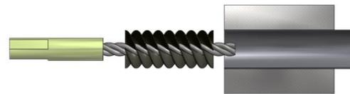
Do not use an oversized brush, force the brush into the tube, or bend the stem. These actions may break the stem and cause deep grooves in the tube. Do not reverse drill because bristles will fall out. A Brush lubricant/Spark inhibitor Lube-A-Tube is available from the factory if required. This should be used when brushing stainless steel tubes or brush may wear out quickly. Brush lubricant / Spark inhibitor should be cleaned from tube before plugging.
