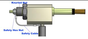
Failure to correctly seat and tighten hydraulic fittings will cause ram piston to lock in extended position after activation.
