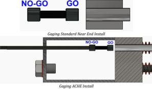
Small end of gage should fit in tube to installation depth and large end should not. For ACHE applications, choose an Extension long enough to reach the tube opening in the tubesheet through the header box. Using an adjacent plug hole as a spotting port or measuring the header box depth and the extension rod to confirm Go/No-Go measurements is helpful.
