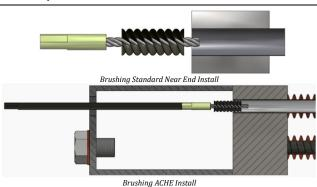
Do not use an oversized brush, force the brush into the tube, or bend the stem. These actions may break the stem and cause deep grooves in the tube. Do not reverse drill because bristles will fall out. A Brush lubricant/Spark inhibitor Lube-A-Tube is available from the factory if required. This should be used when brushing stainless steel tubes or brush may wear out quickly. Brush lubricant / Spark inhibitor should be cleaned from tube before plugging.
