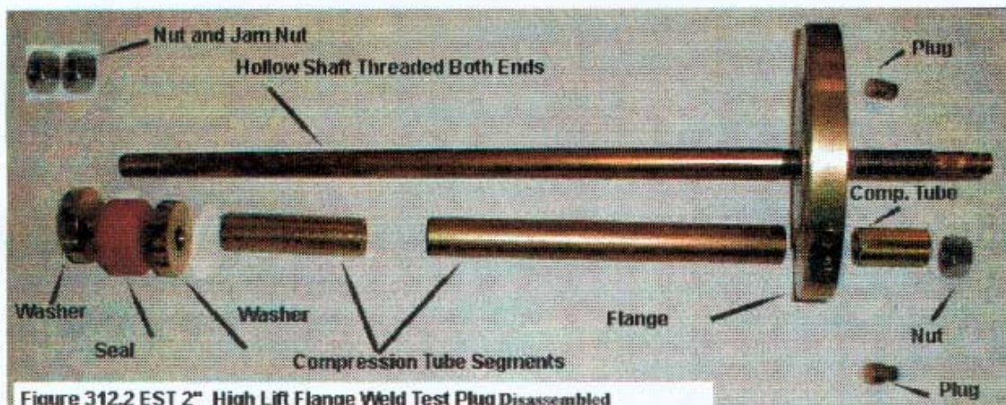
Figure 312.2 EST 2" High Lift Flange Weld Test Plug Disassembled
