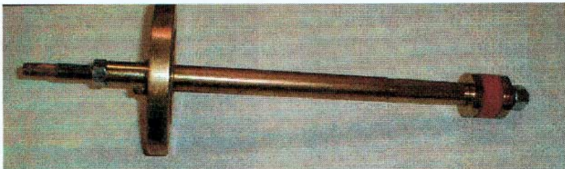
Figure 312.1 EST 2" High Lift Flange Weld Test Plug Assembly
