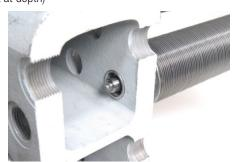
Removal (Easy removal of the installed Pop-A-Plug® in preparation for re-tubing)
