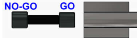
Figure 6A – Second Gaging, Near End Install
