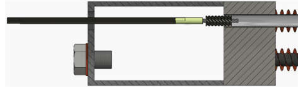
Figure 4B – Brushing ACHE Install
