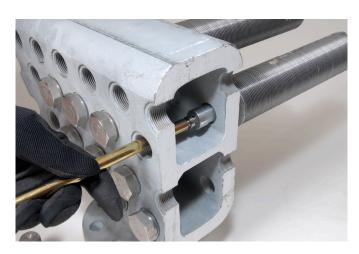
Tube Brushing (Cleaning inside of tube of scale, rust, debris etc. for a clean surface
