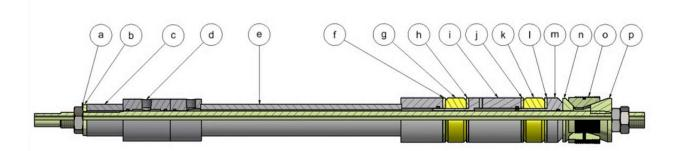
Figure 2: GripTight Isolation Plug Component Parts
