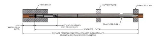
For additional installation and sizing information, please reference: DC1050 -Tube Stabilizer (Rod & CableType) Installation Procedures
