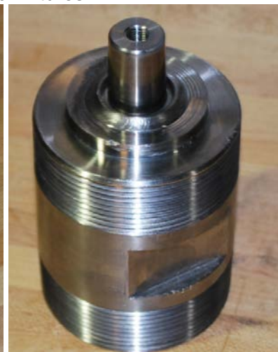
(Fig 14 Machined test coupon with Pop-A-Plug)
