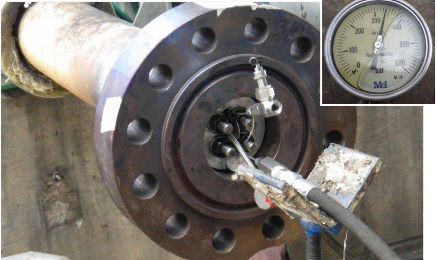
The Double Block & Bleed Isolation Plug at work in the ILBOC refinery
