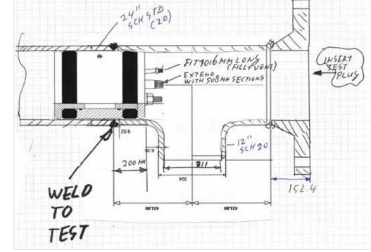
Schematic showing the vertical T section that posed an installation challenge for the DBB plug.
