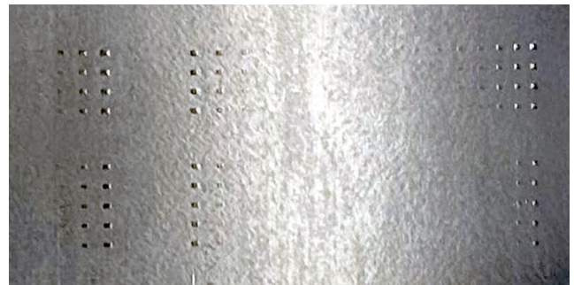
Pic 1. GTMAX Gripper marks in 6" sch 80 pipe at 3,900 psi (276 bar)
