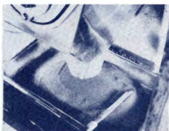
Figure 35. Making the Fuel Rod. This is processed uranium, shown before it is made into fuel pellets.
