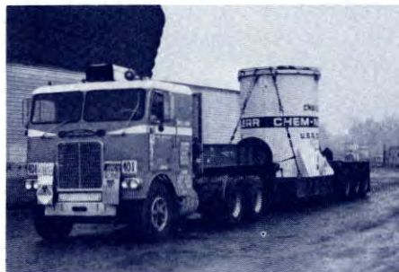
Figure 48. Low Level Waste Shipment. Resins used to filter slightly radioactive water are dried (called dewatering ) and put into these containers for shipment to a disposal area.
