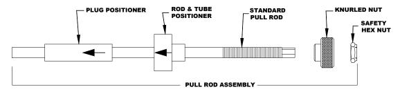
**Note:** The Rod and Tube Positioner for P2-880 and larger plug sizes is a flat washer. It is not stamped with an arrow and may be installed in either direction.
