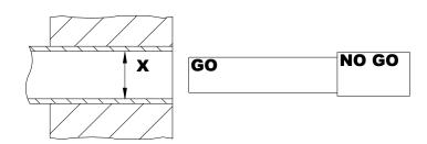
If the Go end of the gage fits, remove the gage from the tube end and attempt to insert the No-Go end of
