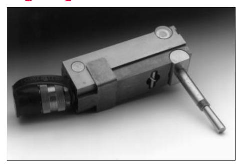
EST's Close Quarters Ram lets you install Pop-A-Plugs even when there's only minimal clearance around the tube end — in the outermost row of tubes in a closed head feedwater heater, for example, or in the tubes adjacent to a
