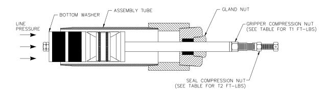
WARNING! LINE PRESSURE MUST ALWAYS PRESSURIZE AGAINST THE BOTTOM WASHER OF THE SEALING ASSEMBLY AS SHOWN ABOVE. NEVER USE TBD VALVE CHANGING TOOL IN REVERSE PRESSURE APPLICATIONS.
